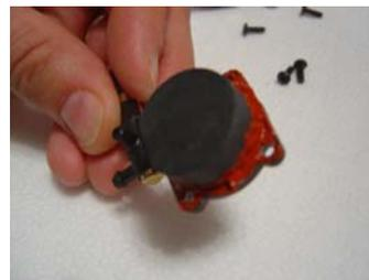
Once the Back Plate is clean and dry, carefully spread red silicon sealer (Wal-Mart and auto parts stores) around the seal of the back plate.
