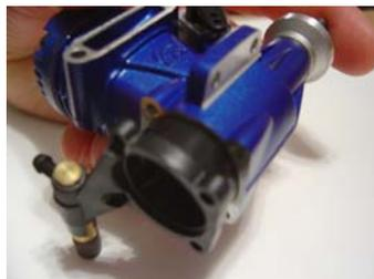
Before you mount the engine, unscrew and remove the back plate using a number 1 Phillips screwdriver. Push hard on the screws so that the heads don't strip. Optionally you can replace the back plate screws with M2.5 x 8 socket head machine bolts, but this isn't necessary.
